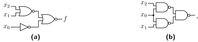
Figure 3: Two different circuits with the minimum gate depth for implementing f = x_0 \wedge (x_1 \vee x_2) used in Example 3.
