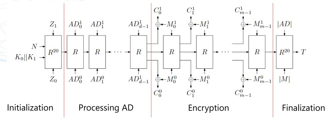
Rocca uses 128-bit nonce, 256-bit key, and output 128-bit tag. The round function absorbs two 128-bit blocks, in total, 256 bits. **Round function of Rocca**
