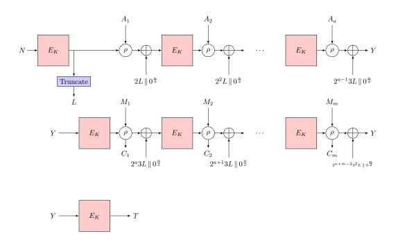
Figure 1: The COFB mode of operation.
