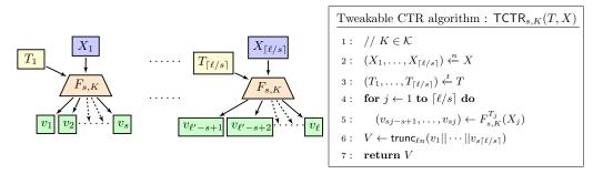
**Figure 5:** Tweakable CTR. This algorithm is parameterized by a multi-forkcipher  $F_s : \mathcal{K} \times \{0,1\}^t \times \{0,1\}^n \to \{0,1\}^{sn}$ . An input vector  $X = \{X_j | 1 \le j \le \lceil \ell/s \rceil\}$  and a tweak vector  $T = \{T_j | 1 \le j \le \lceil \ell/s \rceil\}$  must be provided to generate the output vector V having  $\ell$  *n*-bit blocks. Here  $\ell'$  is defined as  $s \lceil \ell/s \rceil$ .
