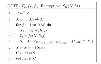
**Figure 2: Encryption algorithm of the generic CTR mode** instantiated with a MFC  $F_s : \mathcal{K} \times \{0,1\}^t \times \{0,1\}^n \to \{0,1\}^{sn}$ . Different definitions of the functions  $f_X$  and  $f_T$  yield concrete variants of the GCTR (see Table 2).
