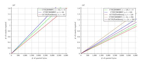
**Figure 4:** Efficiency comparison of any GCTR[ForkSkinny] (with s = 2) with CTR[SKINNY] and CTRT[SKINNY] modes. These plots show the number of rounds required to process the queried bytes  $(sn\sigma/8)$ . The left figure corresponds to the input size n = 64 bits whereas the right figure corresponds to the input size n = 128 bits.
