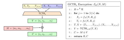
Figure 6:  $GCTR_s$  mode redefined with TCTR. This definition is equivalent with the definition presented in Sect. 4.1.
