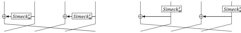
Figure 1: Step Function of sLiSCP (left) and sLiSCP-light (right) Permutations. \text{Simeck}_w^r denotes r -rounds of w -bit block Simeck.
