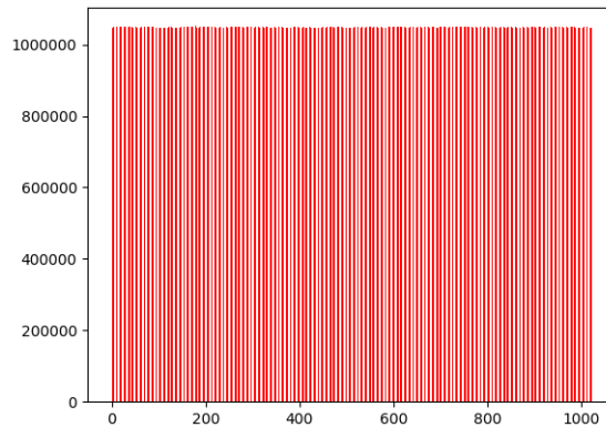
Figure 4: Histogram plotting how many times each of the 2^{10} possible two successive input of the function h were reached after 2^{30} Grain v1 initialization using random key and iv values.
