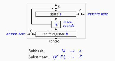
b: 256-bit shift register with 32-bit stages
