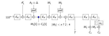
4.  $\mathcal{A}$  makes query  $\mathcal{E}_{\mathcal{K}}(\mathcal{A}'[1] || (\mathcal{A}[2] \oplus \Delta) || \mathcal{A}[3] || \dots || \mathcal{A}[a], \mathcal{M}))$  and obtains (C, T),  $\Delta = \mathcal{M}_2[1] \oplus \mathcal{C}_2[1] \oplus \mathcal{M}_3[1] \oplus \mathcal{C}_3[1]$ .
