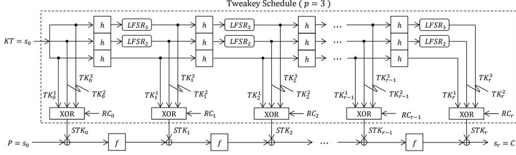
**Figure 1:** Tweakey schedule and encryption process of Deoxys-BC-384 [CHP<sup>+</sup>17]
