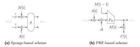
**Figure 2: (a)** The Sponge-based scheme with full absorption [SY15, MRV15]. p is a public permutation. **(b)** The PRF-based scheme with full absorption [RVV15].  $F_K$  is a PRF and  $\Delta$  is a mask that depends on the key, nonce, and the block counter. These schemes are non-parallelizable, and full absorption is achieved by utilizing the chaining values.
