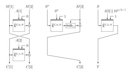
**Figure 33:** The encryption process of a plaintext  $M = (M[1], M[2], M[3]) \in \{0, 1\}^{3n}$ and AD  $A = (A[1], A[2], A[3]) \in \{0, 1\}^{2.5n}$  with iZOTR. The output is a ciphertext C = (C[1], C[2], C[3]) and a tag T. S is  $M[2] \oplus M[3]$ .
