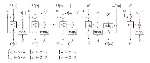
**Figure 18:** Core.Enc<sub>K</sub>(N, B, M) of ZOCB, where  $(B[1], \ldots, B[m]) \xleftarrow{t} B$ . The value of  $\nu$  in the last step is 1 if  $|M[m]| \neq n$  and 2 otherwise. S is  $M[1] \oplus \cdots \oplus M[m-1] \oplus \mathsf{ozp}_n(M[m])$ .
