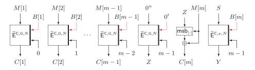
**Figure 4:** iCore.Enc<sub> $\widetilde{\mathsf{E}}$ </sub>(N, B, M) of iZOCB, where  $(B[1], \ldots, B[m]) \xleftarrow{t} B$ . The value of  $\nu$  in the last step is 1 if  $|M[m]| \neq n$  and 2 otherwise. S is  $M[1] \oplus \cdots \oplus M[m-1] \oplus \mathsf{ozp}_n(M[m])$ . The red dashed lines are t bits wide (also in other figures).
