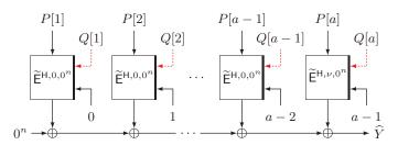
**Figure 5:** iHash<sub> $\widetilde{E}$ </sub>( $\widehat{B}$ ) of iZOCB, where ( $\widehat{B}[1], \ldots, \widehat{B}[a]$ )  $\xleftarrow{n+t} \widehat{B}$  and (P[i], Q[i])  $\xleftarrow{n,t} \widehat{B}[i]$ .  $\nu$  in the last step is 1 if  $|\widehat{B}[a]| \neq n + t$  and 2 otherwise.
