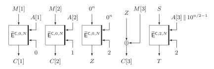
**Figure 31:** The encryption process of a plaintext  $M = (M[1], M[2], M[3]) \in \{0, 1\}^{3n}$ and AD  $A = (A[1], A[2], A[3]) \in \{0, 1\}^{2.5n}$  with iZOCB to produce the ciphertext C = (C[1], C[2], C[3]) and the tag T. S is  $M[1] \oplus M[2] \oplus M[3]$ .
