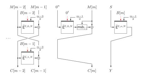
**Figure 12:** iCore.Enc<sub> $\widetilde{\mathsf{E}}</sub>(N, B, M)$  of iZOTR for the case  $m \mod 2 = 1$ . This processes  $M[m-2], \ldots, M[m]$  and  $B[m-2], \ldots, B[m]$ , where  $(B[1], \ldots, B[m]) \xleftarrow{t} B$ .  $\nu$  in the last step is 4 if  $|M[m]| \neq n$  and 5 otherwise. S is  $M[2] \oplus M[4] \oplus \cdots \oplus M[m-1] \oplus \mathsf{ozp}_n(M[m])$ .</sub>
