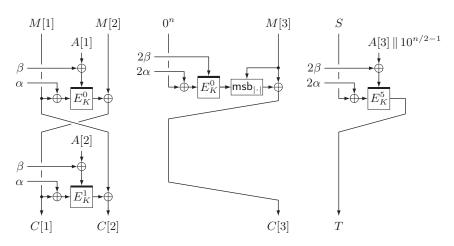
**Figure 34:** The encryption process of  $M = (M[1], M[2], M[3]) \in \{0, 1\}^{3n}$  and  $A = (A[1], A[2], A[3]) \in \{0, 1\}^{2.5n}$  with ZOTR to produce C = (C[1], C[2], C[3]) and  $T. \alpha = E_K^{6,0^n}(N), \beta = E_K^{6,0^{n-1}1}(N)$ , and  $S = M[2] \oplus M[3]$ .
