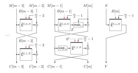
**Figure 11:** iCore.Enc<sub>E</sub>(N, B, M) of iZOTR for the case  $m \mod 2 = 0$ . This illustrates the process of  $M[m-3], \ldots, M[m]$  and  $B[m-3], \ldots, B[m]$ , where  $(B[1], \ldots, B[m]) \xleftarrow{t} B$ .  $\nu$  in the last step is 2 if  $|M[m]| \neq n$  and 3 otherwise. S is  $M[2] \oplus M[4] \oplus \cdots \oplus M[m-2] \oplus ozp_n(C[m]) \oplus Z$ .
