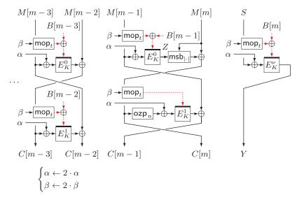
**Figure 27:** Core.Enc<sub>K</sub>(N, B, M) of ZOTR for the case  $m \mod 2 = 0$ . This illustrates the process of  $M[m-3], \ldots, M[m]$  and  $B[m-3], \ldots, B[m]$ , where  $(B[1], \ldots, B[m]) \stackrel{t}{\leftarrow} B$ .  $\nu$  in the last step is 2 if  $|M[m]| \neq n$  and 3 otherwise. S is  $M[2] \oplus M[4] \oplus \cdots \oplus M[m-2] \oplus \mathsf{ozp}_n(C[m]) \oplus Z$ .
