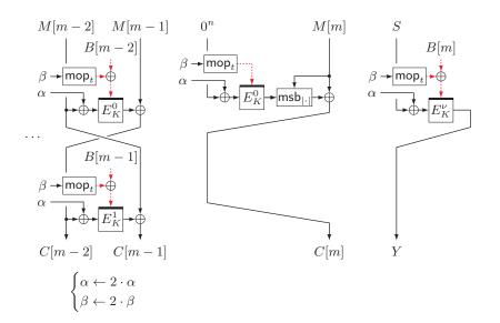
**Figure 28:** Core.Enc<sub>K</sub>(N, B, M) of ZOTR for the case  $m \mod 2 = 1$ . This processes  $M[m-2], \ldots, M[m]$  and  $B[m-2], \ldots, B[m]$ , where  $(B[1], \ldots, B[m]) \stackrel{t}{\leftarrow} B$ .  $\nu$  in the last step is 4 if  $|M[m]| \neq n$  and 5 otherwise. S is  $M[2] \oplus M[4] \oplus \cdots \oplus M[m-1] \oplus \mathsf{ozp}_n(M[m])$ .
