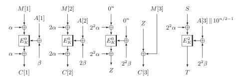
**Figure 32:** The encryption process of  $M = (M[1], M[2], M[3]) \in \{0, 1\}^{3n}$  and  $A = (A[1], A[2], A[3]) \in \{0, 1\}^{2.5n}$  with ZOCB to produce C = (C[1], C[2], C[3]) and  $T. \alpha = E_K^{3,0^n}(N), \beta = E_K^{3,0^{n-1}1}(N)$ , and  $S = M[1] \oplus M[2] \oplus M[3]$ .
