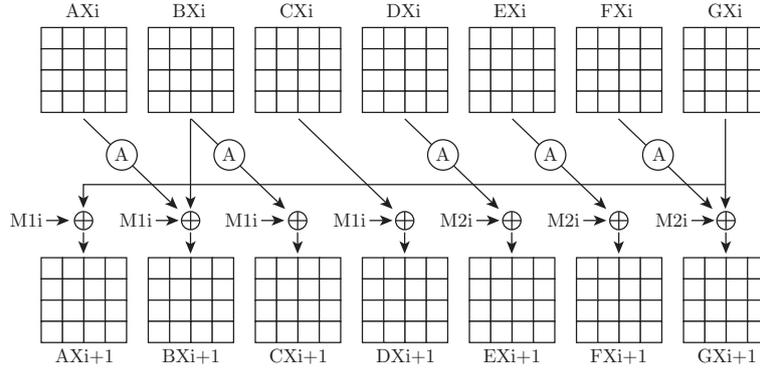
Figure 2: C5 construction. ‘A’ represents AES round function.
