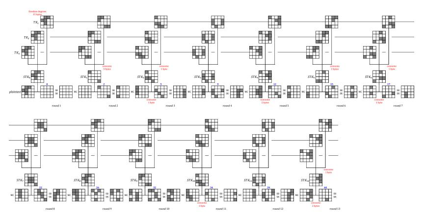
**Figure 5:** A 13-round truncated differential path considering degrees. Red comments explain the evaluation of degrees and blue numbers count the active S-boxes.
