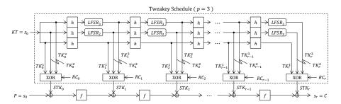
Figure 1: Instantiation of the TWEAKEY framework for Deoxys-BC-384.
