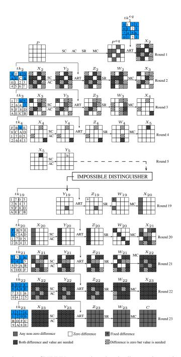
Figure 6: 23-round attack against SKINNY-n-2n. The colored cells in each round tweakeys represent the cells, the values for which should be known to verify the differential path. During our attack, some of these tweakey cells are guessed and some of them are derived from the information that we have at each step of the attack.
