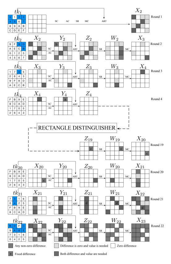
Figure 9: Tweakey rovery attack on 22-round SKINNY-64-128
