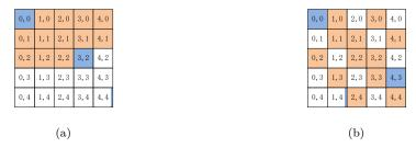
Figure 18: Initialize State with Key, Padding and Nonce in Ketje Jr v1 (a) and v2 (b)
