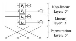
Figure 6: Extended Generalized Feistel Network.
