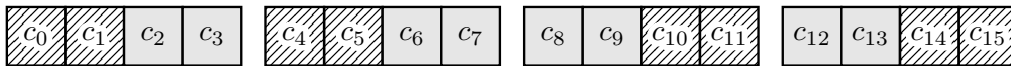
Figure 2: Truncation in Haraka-512/256 : the dashed columns are truncated away. Each column c_i contains four bytes.
