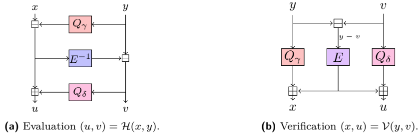
Figure 1: Nonlinear layer of the Anemoi round function: Open FLYSTEL \mathcal{H} : \mathbb{F}_q^2 \rightarrow \mathbb{F}_q^2 for evaluation (high-degree) and closed FLYSTEL \mathcal{V} : \mathbb{F}_q^2 \rightarrow \mathbb{F}_q^2 for verification (low-degree).
