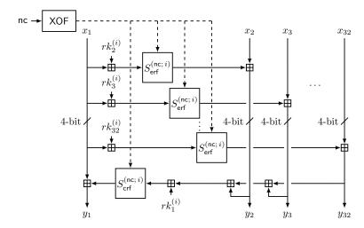
**Figure 2:** The *i*-th round function of FRAST.  $rk_1^{(i)}, \ldots, rk_{32}^{(i)}$  are the *i*-th round keys.
