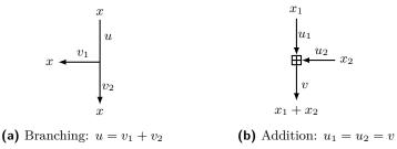
Figure 5: Linear masks for branching and addition
