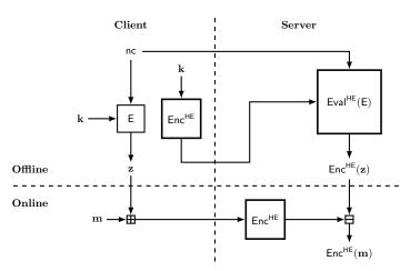
**Figure 1:** The transciphering framework with a stream cipher. Homomorphic operations are performed in the boxes with thick lines. The vertical dashed line distinguishes the client and server, and the horizontal dashed line distinguishes the offline and online computations. The encryption Enc<sup>HE</sup> performed by the server in the online phase can be done trivially. nc is a public nonce.
