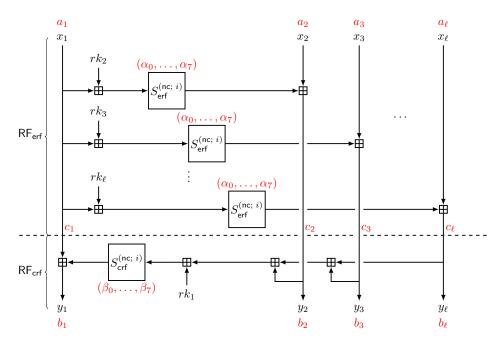
Figure 6: Linear masks in a single round of the FRAST considering XOF.
