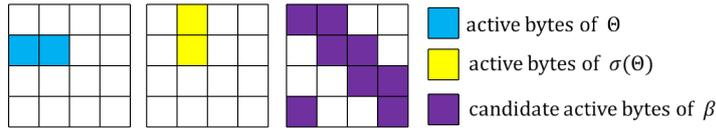
**Figure 4:** An example when  $\Theta$  has two active bytes located in the same row
