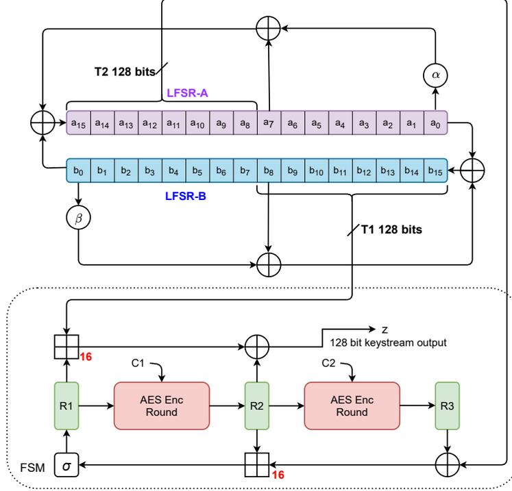
**Figure 1:** The schematic of SNOW 5G
