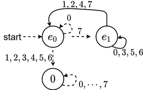
**Figure 2:** The automaton for the modular addition with two inputs
