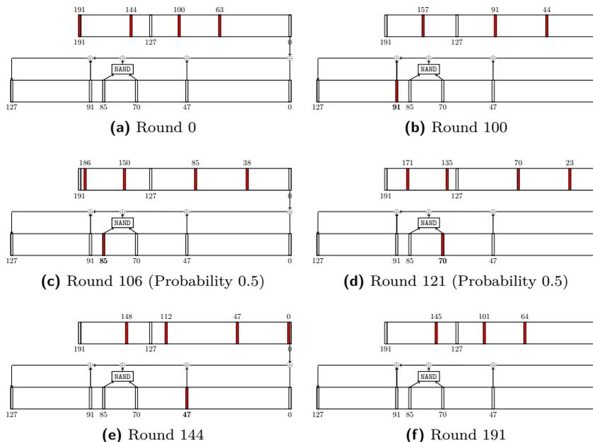
**Figure 6:** The iterative differential characteristic for TinyJAMBU with a 192-bit key. The rounds are modulo 192.
