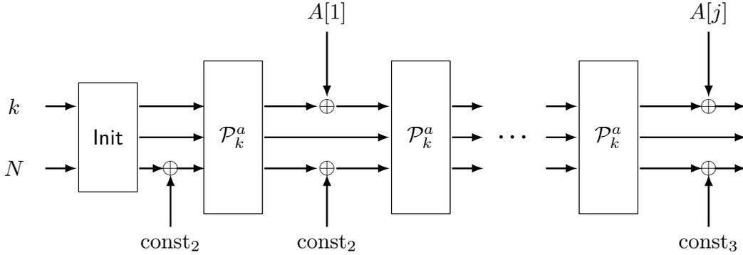
Figure 3: Processing the associated data.
