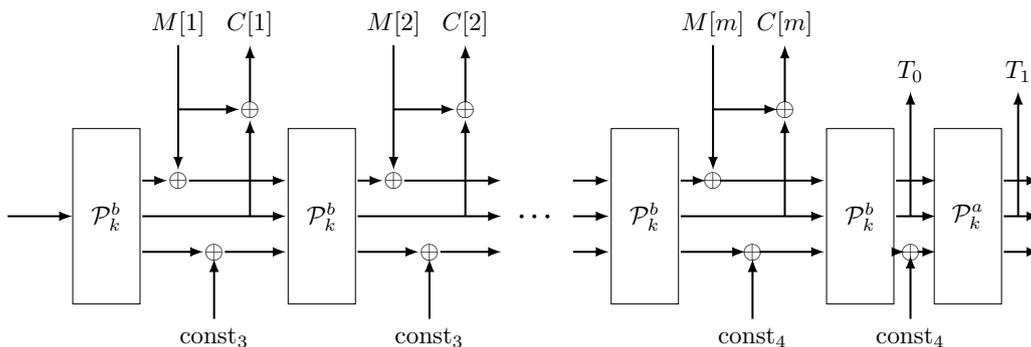
Figure 4: TinyJAMBU encryption and finalization.
