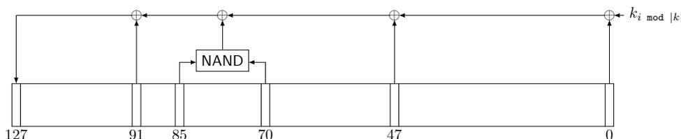
**Figure 1:** Round function of the TinyJAMBU permutation.
